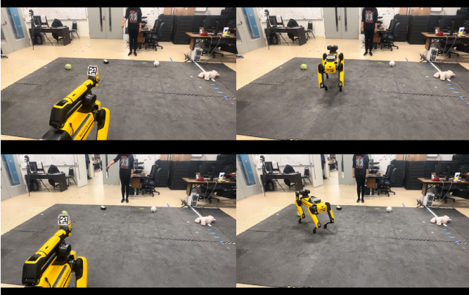
Fig. 3: Our system enables the robot to correctly fetch the object the human user is pointing at, such as the penguin plush (left) and green cat (right).
