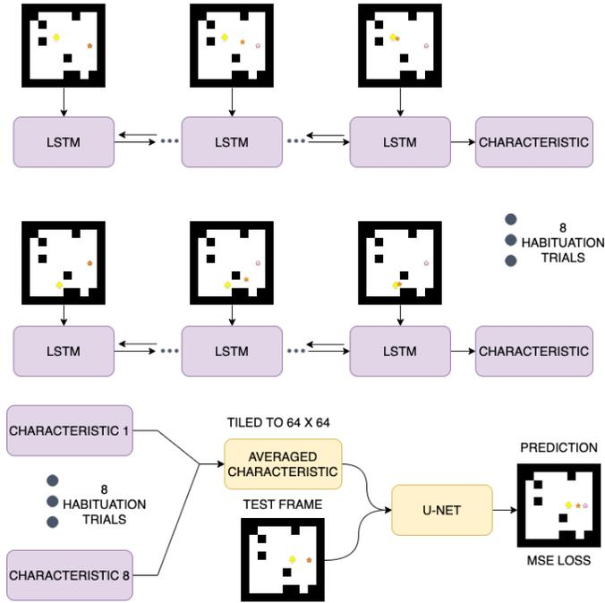
Fig. 7: Architecture of the video baseline model inspired by Rabinowitz et al. (2018) [34]. An agent-characteristic embedding is inferred from the familiarization trials using a recurrent net. This embedding, with the state at test time, is used to predict the next frame of the video using a U-Net [39].
